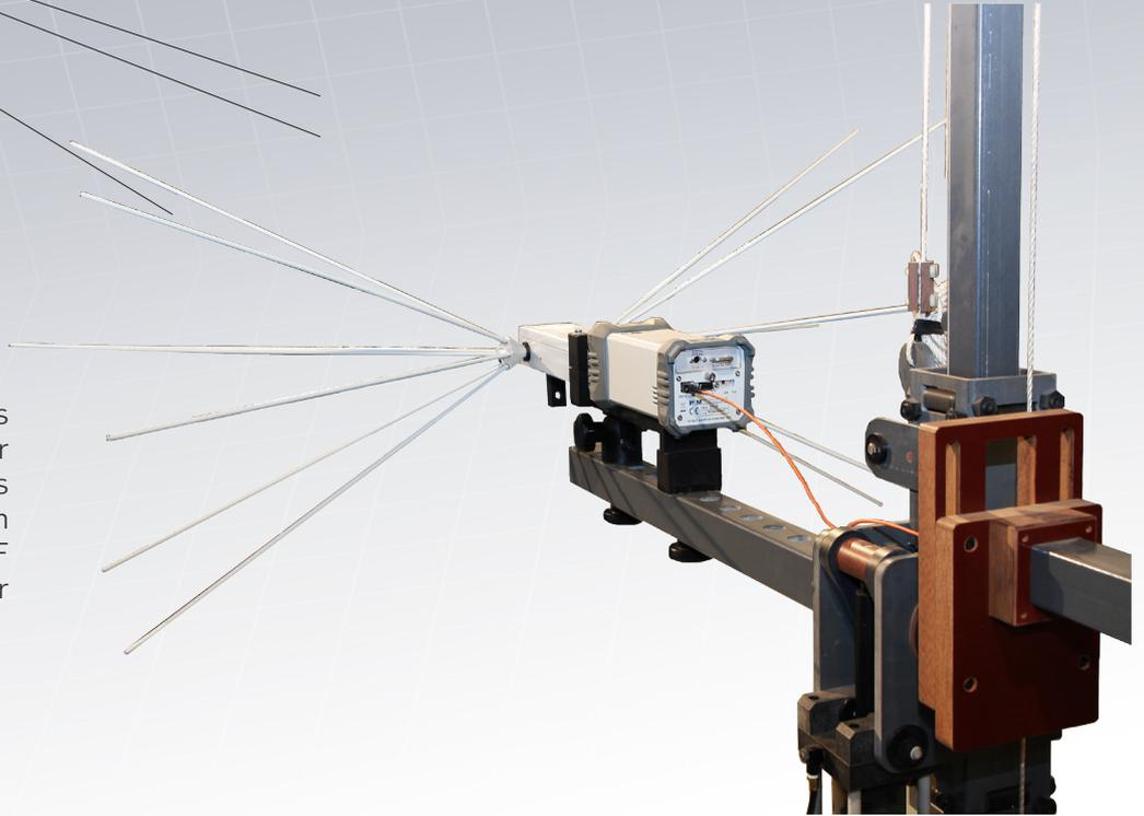
**IEC/EN 55015:** radiated measurement with the Large Loop Antenna easier and faster than never thanks to the high-speed of 9010F in conjunction with the RF switch SBRF4 automatically switching the x-y-z axis.
