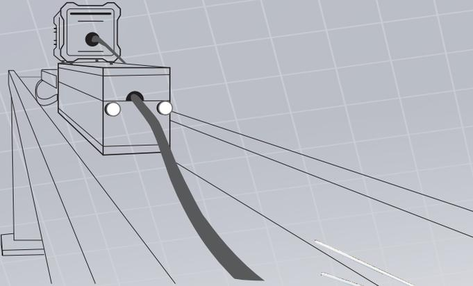
The set of mounting adapters supplied with PMM's Receiver Modules is suitable for several types of antennas: its special design avoids mechanical stress to the RF connectors and allows for an easier installation on the antenna pole.
