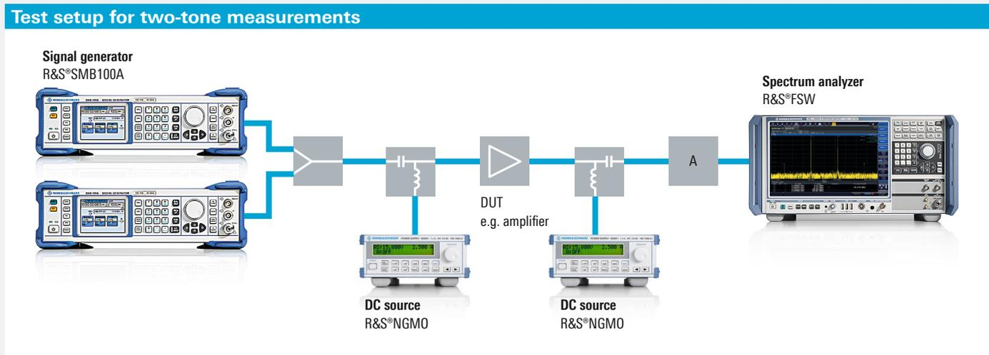
The test setup consists of two R&S®SMB100A signal generators, an R&S®FSW signal and spectrum analyzer for displaying the results, and two R&S®NGMO DC sources for setting the gate and drain voltage.
