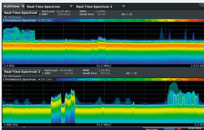
Simultaneous display of two spectra in the 512 MHz wide persistence spectra with the R&S®FSW MultiView function: ISM band at 2.4 GHz (top); mobile communications signals at 2.1 GHz and ISM band at 2.4 GHz (bottom).
