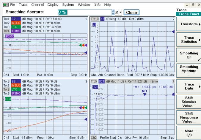
Intermodulation measurements on an amplifier in pulsed mode.
