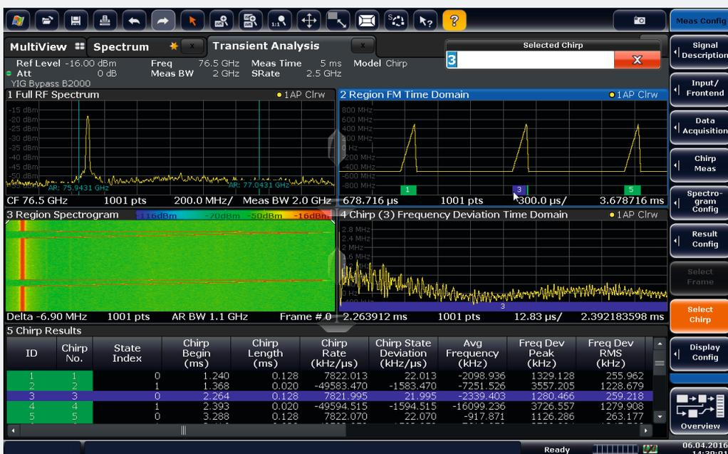
Analysis of a 2 GHz wide chirp signal at 76.5 GHz using the R&S®FSW-K60/K60C measurement options.
