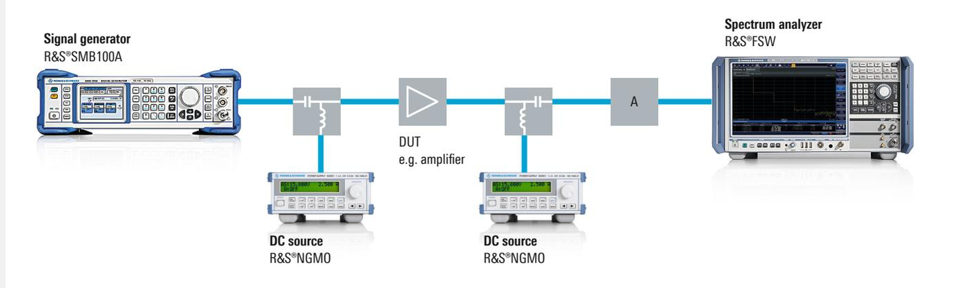
The test setup consists of an R&S®SMB100A signal generator, an R&S®FSW signal and spectrum analyzer for displaying the results, and two R&S®NGMO DC sources for setting the gate and drain voltage. Very high output powers require the use of an additional attenuator (A) to protect the spectrum analyzer's input port.
