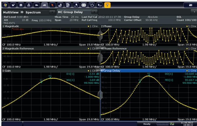
Intuitive touchscreen operation: example of reference and DUT measurement with bandpass characteristic using the R&S®FSW.
