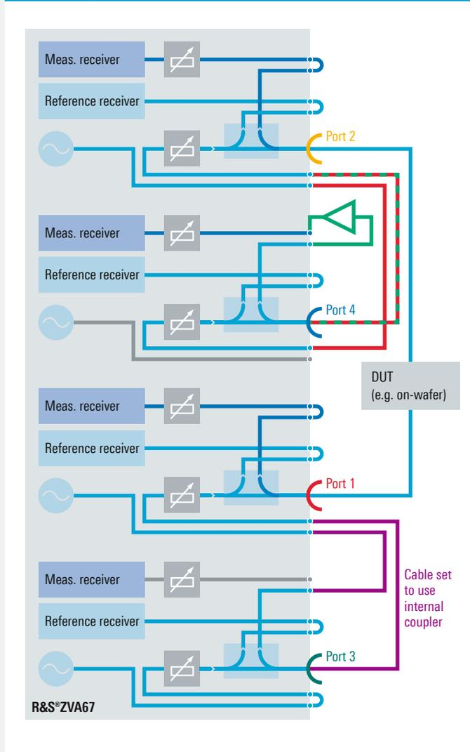
A two-tone signal for the intermodulation measurement is generated at port 1. Port 2 is used as a receiver port. The noise figure is measured at port 4 in order to loop in a pre-amplifier for DUTs with low gain. All measurements use the same probe contacts, making results comparable and speeding up measurements.
