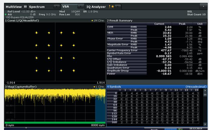
Modulation analysis of a 1.8 GHz bandwidth 16QAM signal with the R&S®FSW-K70 option: various graphs and tables provide information about the modulation quality at a glance.
