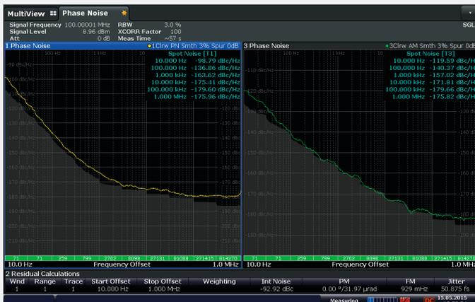
The R&S®FSWP measures phase noise (left) and amplitude noise (right) simultaneously: the gray area shows the correlation gain of the R&S®FSWP; if the gray area is clearly below the trace, the DUT is measured and the sensitivity is not limited by the local oscillator.
