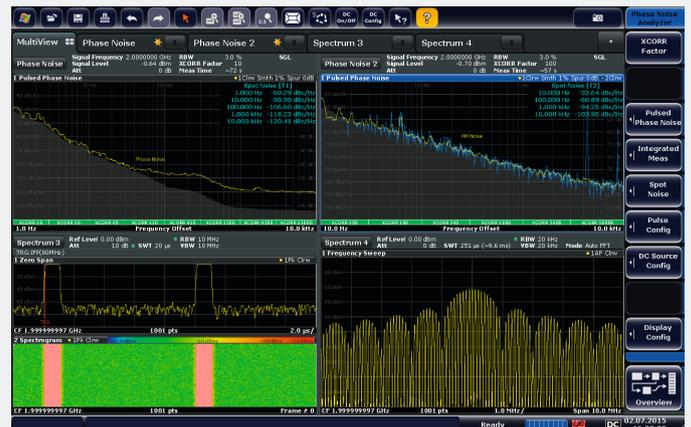
Pulsed signal measurement in time and frequency domain using the R&S®FSWP spectrum analyzer function: phase noise of pulsed source up to an offset equal to one half of the pulse repetition rate (upper left) and amplitude noise (upper right).
