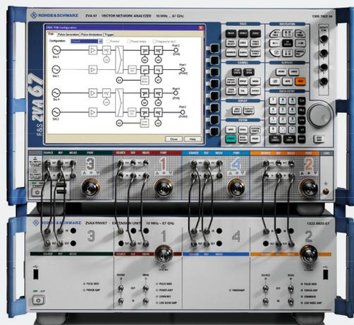
Test solution consisting of R&S®ZVA and R&S®ZVAX-TRM.
