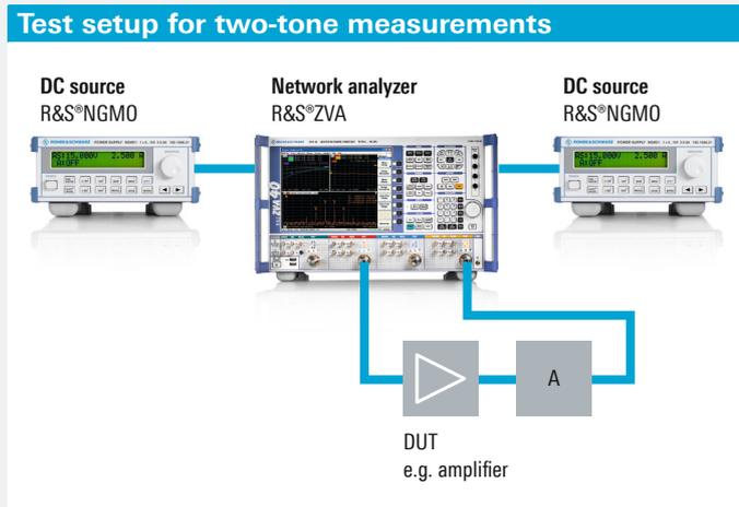
The test setup consists of an R&S®ZVA vector network analyzer for generating the two-tone signal at port 1 and for displaying the results, and two R&S®NGMO DC sources for setting the gate and drain voltage via the internal R&S®ZVA bias tees.
