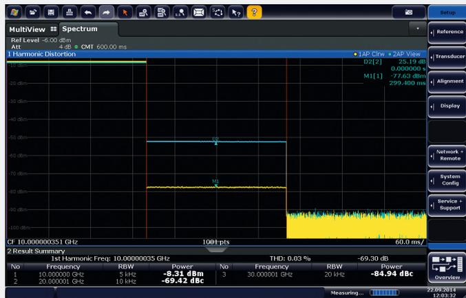
Benchmark measurement of amplifier harmonics (fundamental, first and second harmonic) using the R&S®FSW. When the R&S®SMB100A internal low harmonic filter is activated (yellow), measurement accuracy can be increased by approx. 25 dB.
