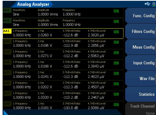
Figure 1. The U8903B's GUI, showing 8 analyzer channel measurements.
