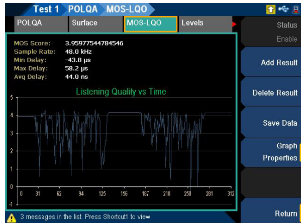
Figure 4. The MOS (Mean Opinion Score) scoring, indicating the rating of the DUT's voice quality.
