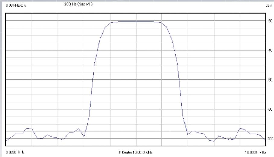
After the A/D conversion the behaviour of a regular receiver is mathematically simulated in order to perfectly match international standards specifications. Even for a digital architecture, preselector filters and input attenuators are mandatory for limiting the signal energy into well defined RF bands, to improve the dynamic range and to increase the signal to noise ratio, thus ensuring accurate measurements of all wideband complex signals typical of EMC measurements.
