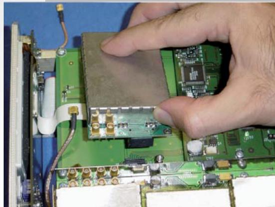
Moreover, the outstanding feature that service can be easily done by simply replacing plug-in pre-calibrated subassemblies, represents a highly valued advantage in case, for example, of damage to the RF front-end. Indeed, even when an excess of energy
