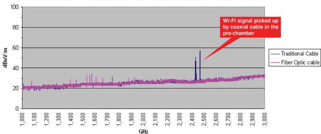
Comparison between antenna-receiver connected by coaxial cable (blue trace) and 9030 directly connected to the antenna and linked to 9010 by fiber optic cable (pink trace). The example shows how PMM's solution can prevent unwanted signals being picked up by the coaxial cable along its path from the antenna to outside the chamber.
