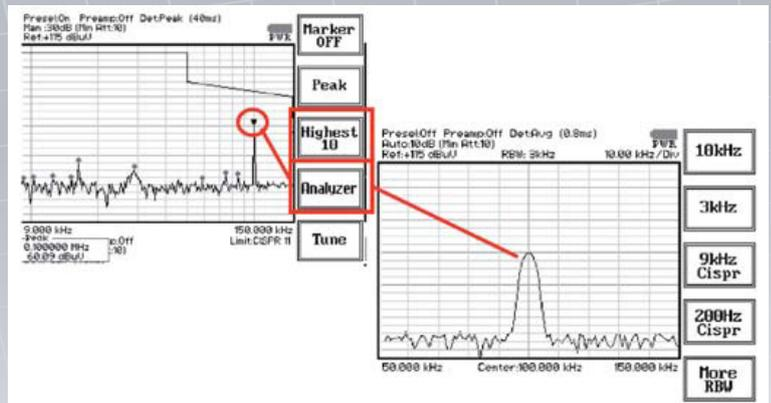
The 9010 features several useful functions: as an example, pictures above show the automatic highest peaks finder and the intuitive way to observe the selected peak in Analyzer mode: from measurement to debugging at users' fingertips!
